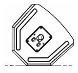
The rear side inclination, symmetrical, as shown in the upper picture, is 45°. SYA12 can be used as a stage monitor in small contexts, in this case please consider the characteristic dispersion pattern presented above.
